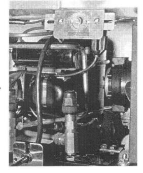
Removal of louvre grill exposes motor and temperature control. Counterclockwise for warmer or clockwise for colder, as necessary. Typical range is 0°to -20° (F)
