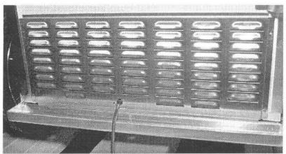
For Temperature adjustment, machine louvre grill is to be removed. Grill located under handle-bar.
