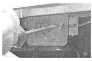
For further adjustment warmer, remove thermostat control by removing screws retaining control to mounting bracket.
